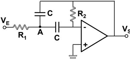
$$\frac{V_s(p)}{V_e(p)} = - \frac{\frac{p}{R_1 C}}{p^2 + 2 \frac{p}{R_2 C} + \frac{1}{R_1 R_2 C^2}}$$
